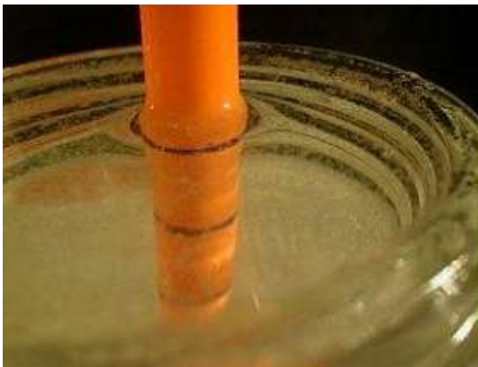
Figure 5.07: Meniscus correction to the actual hydrometer reading.
